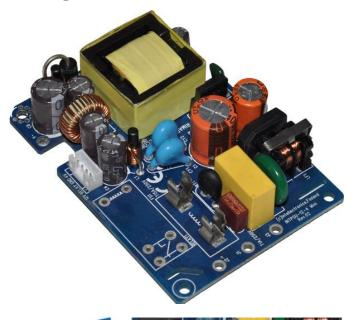
PSU with pre-installed fuse brackets, no relay, no fuse. or
