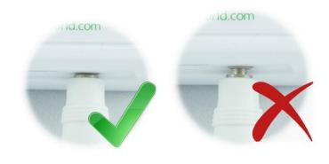
NOTE! Check that the sensor is inserted all the way into the 3.5mm red jack socket right to the very end. You must ensure that there is no gap between the connector of the sensor and the jack socket. Do NOT apply excessive force!
