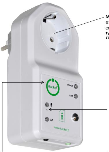
**Hidden button:** used to switch the main socket manual (Chapter 4.3) or reset device (Chapter 15).
